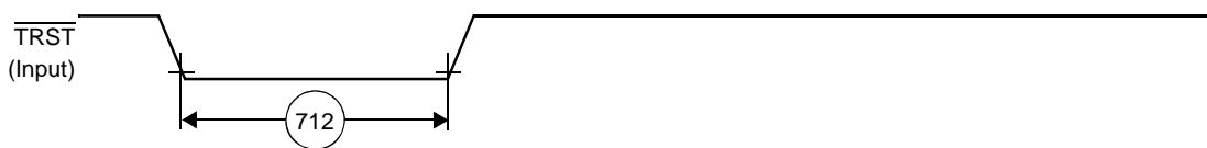
Figure 29. TRST Timing Diagram
