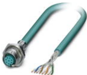
Bus system flush-type socket, Ethernet, 8-pos., M12, shielded, rear/screw mounting with M16 thread, with 0.5 m bus cable, 4 x 2 x 0.26 mm 2
