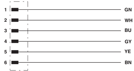
Contact assignment of 7/8" plug
