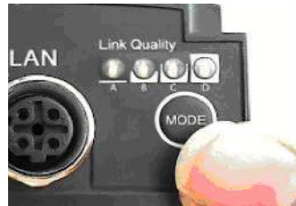
Figure 2-1 “MODE” button on the bottom of the FL WLAN EPA - Above the “MODE” button are LEDs “A” to “D” for configuration indication
