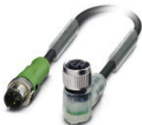
Sensor/actuator cable, 3-position, Variable cable type, Plug straight M12 SPEEDCON, A-coded, on Socket angled M12 SPEEDCON, A-coded, with 2 LEDs, cable length: Free input (0.2 ... 40.0 m)
