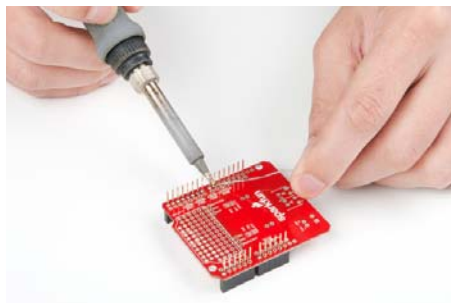
In the process of soldering stackable headers. Still a lot of pins to go!
