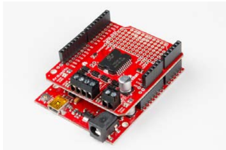
Ardumoto Shield assembled and situated on a RedBoard.
