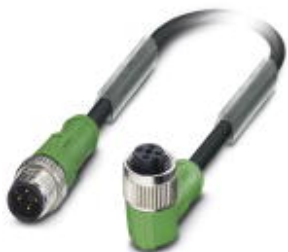
Sensor/actuator cable, 4-position, PUR halogen-free, black-gray RAL 7021, Plug straight M12, A-coded, on Socket angled M12, A-coded, cable length: 5 m
