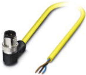
Sensor/Actuator cable, 3-position, TPE, yellow RAL 1021, Plug angled M12 SPEEDCON, A-coded, on free cable end, Cable length: 2 m
