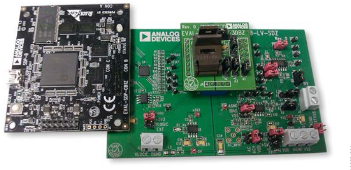
Figure 1. Digital Picture of Evaluation Board with Low Voltage DigiPOT Motherboard and System Demonstration Platform
