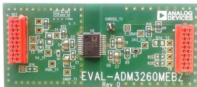
Figure 1. EVAL-ADM3260MEBZ Evaluation Board
