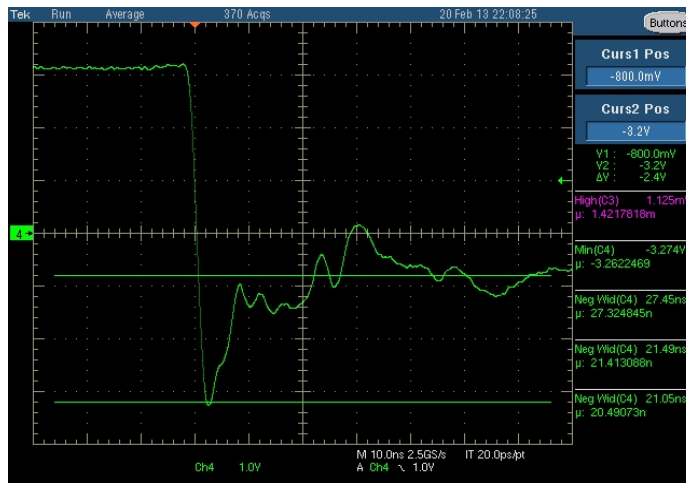
Figure 4. Typical Reverse Recovery I_F = 750 \text{ mA} to V_R = 36 \text{ V}
