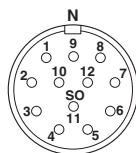
Pin assignment M23 socket, 12-pos., female side view
