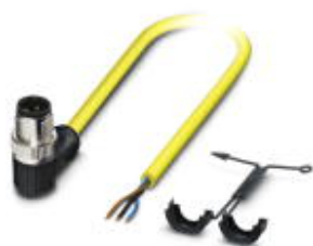
Sensor/Actuator cable, 3-position, PVC, yellow, Plug angled M12 SPEEDCON, A-coded, on free cable end, Cable length: 5 m
