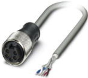
Bus system cable, DeviceNet, 5-position, PUR halogen-free, Gray RAL 7001, Free cable end, on Socket straight 7/8"-16UNF, Cable length: 10 m
