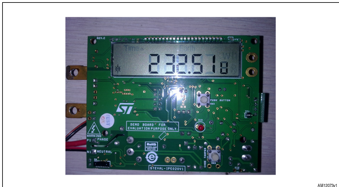
Figure 1. Single-phase energy meter solution based on STPM10 and STM8L152C6 with dual interface EEPROM
