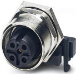
Sensor/actuator flush-type connector, socket, 5-pos., M12, A-coded, rear/screw mounting with M12 thread, with polarity protection, with angled solder connection
