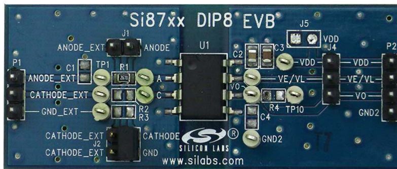
Figure 1. Si871x DIP8 Evaluation Board Overview
