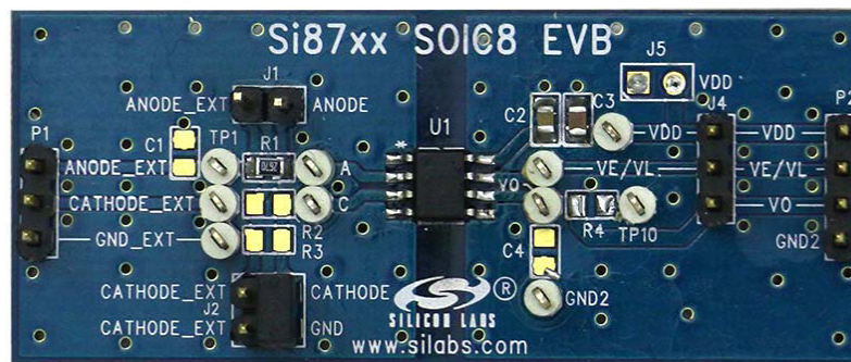
Figure 2. Si871x SOIC8 Evaluation Board Overview
