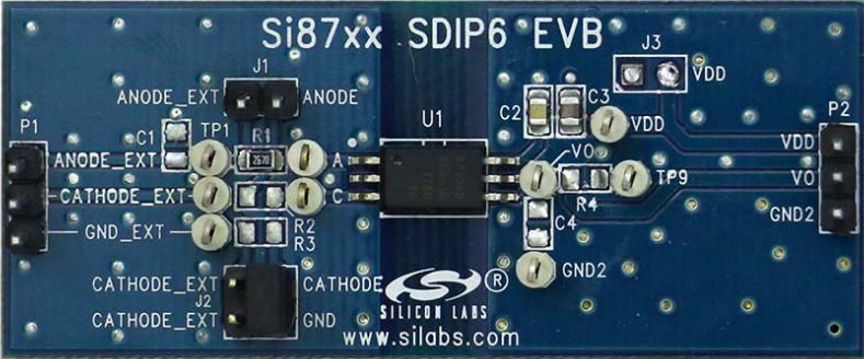
Figure 3. Si871x SDIP6 Evaluation Board Overview
