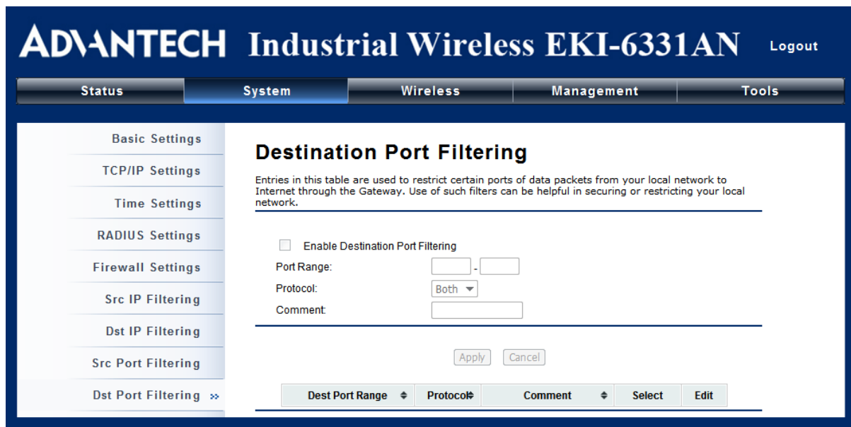
Figure 19 Destination Port Filtering
