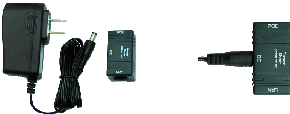
Figure 5 Connect to POE Injector
