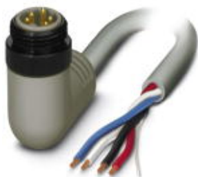
Bus system cable, DeviceNet™, 5-position, PVC, gray, Plug angled 7/8"-16UNF, on free cable end, cable length: 2 m
