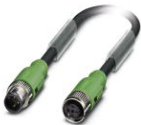
Sensor/actuator cable, 3-position, Variable cable type, shielded, Plug straight M12 SPEEDCON, A-coded, on Socket straight M12 SPEEDCON, A-coded, cable length: Free input (0.2 ... 40.0 m)
